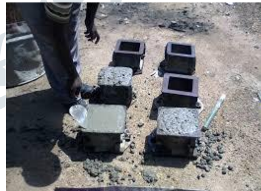
Fig 5. Casting of cubes with vibrator
