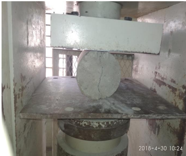
Fig 8 Testing of cylinder by split tensile strength
