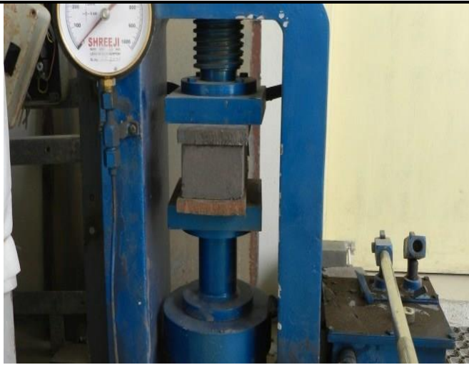
Fig 7 Testing of cube
