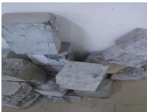
Figure -3: Tested concrete cubes
