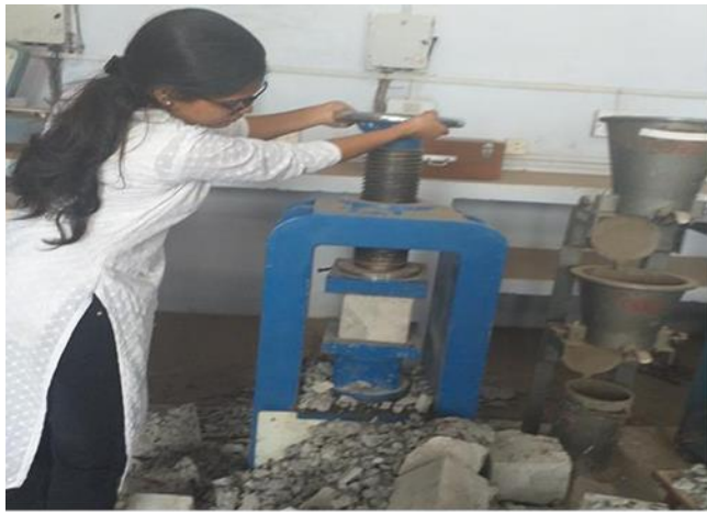
Fig.7.1 compression strength test cube specimen
