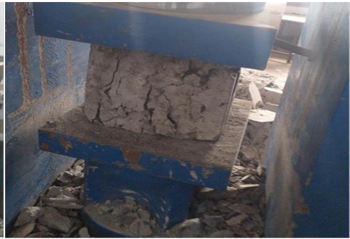
Fig.7.2 cube specimen after loading
