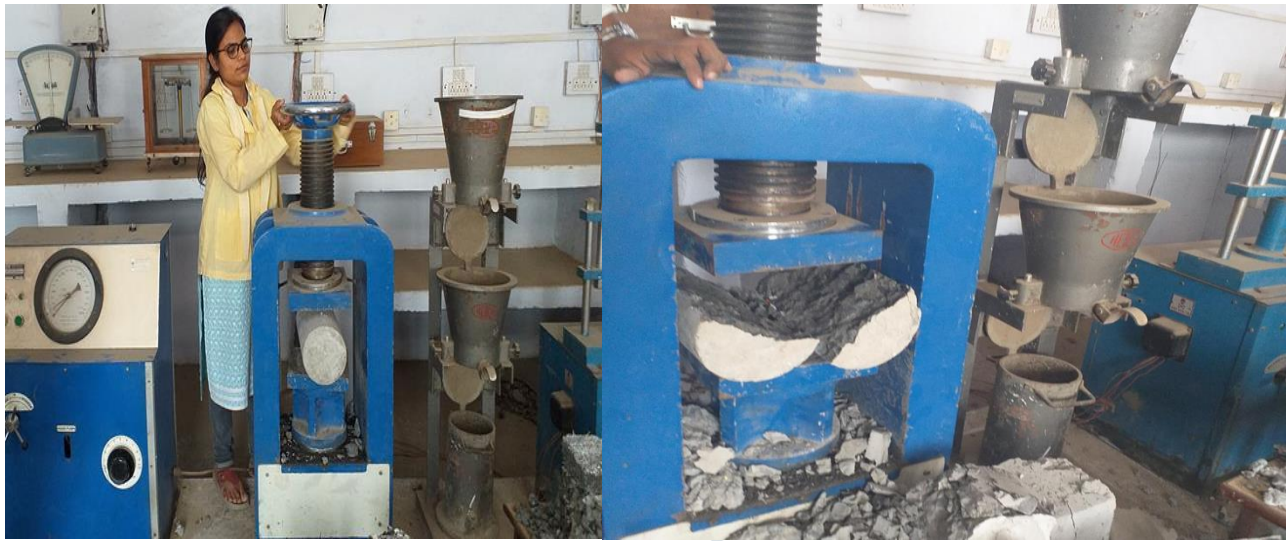
Fig.7.3 Testing of cylinder specimen
