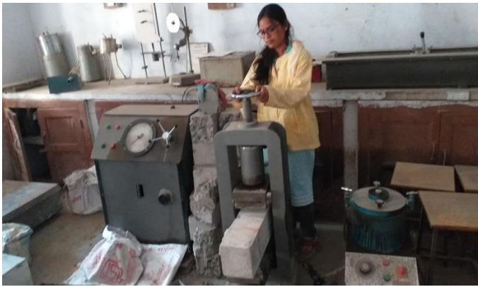
Fig.7.5 Shows Testing of Beam Specimen
