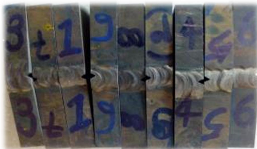
Fig 5.1: Schematic sketch of Charpy impact test specimens
