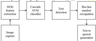
a bus detection and recognition system is proposed, the system is able to recognize coming bus route and other text and generate speech to the visually impaired user, the bus detection is done by using HOG descriptor and cascade SVM classifier as shown in and then text detection and recognition algorithm come into picture, its output goes to text to speech generation engine. A clothing pattern recognition prototype system is developed in [18], this system is able to recognize four clothing
