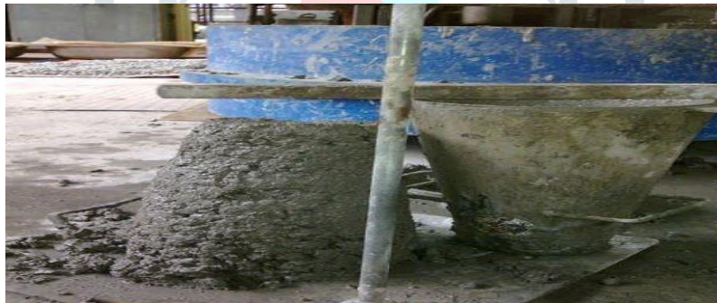
Fig.5: Slump Test Result
