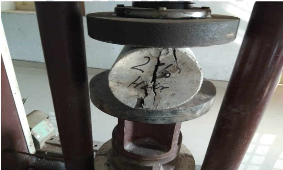
Fig. 12: Split Tensile Strength Test
