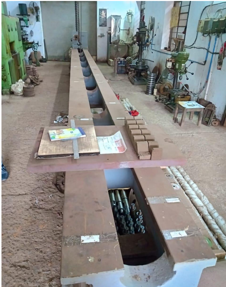
Fig. 5: Real Snap of Base Structure of Deep Hole Boring Machine
