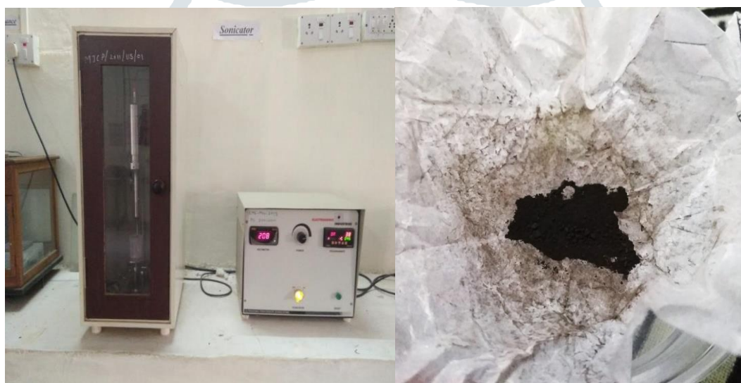
Figure 3(a) & (b): Probe-sonicator and final product of MnO 2 nanoparticles
