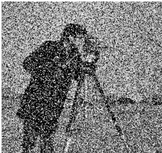
Fig. 7: Watermarked image under salt and pepper noise attack (intensity= 0.4)
