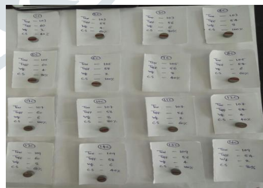
Fig.5 Circular profile machined workpieces
