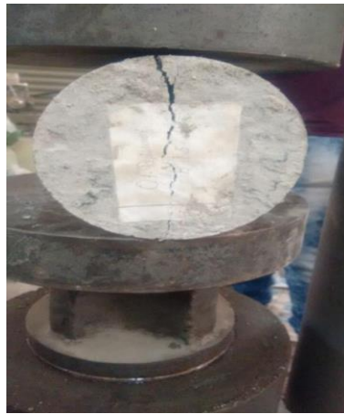
Fig 7. Testing of concrete cube in compression testing machine
