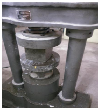
Fig 5. Testing of concrete cube in compression machine
