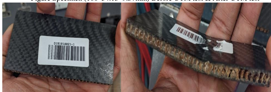
Figure 7.2 Specimen (100*54.13*6.72mm) Before UTM test & After UTM test
