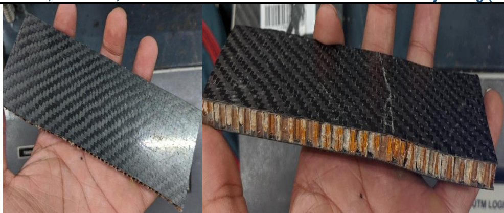
Figure 7.3 Specimen (150*56.57*9.43mm) Before UTM test & After UTM test
