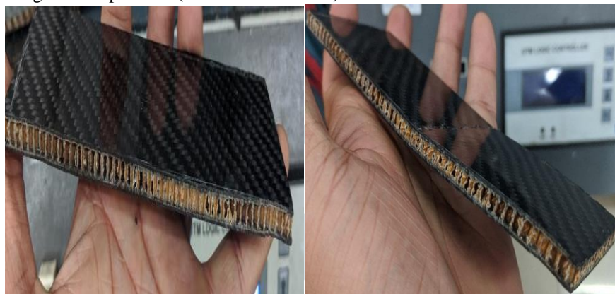
Figure : Specimen (150*55.15*6.72mm) Before UTM test & After UTM test
