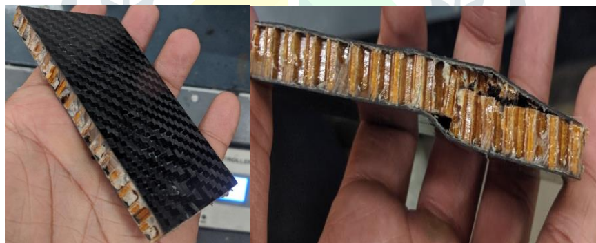
Figure Specimen (100*54.13*9.37mm) Before UTM test & After UTM test
