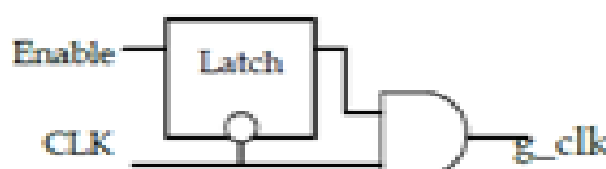
Fig.1 Latch based Clock gating Cell
