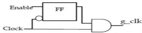
Fig. 2 Flip flop based clock gating Cell
