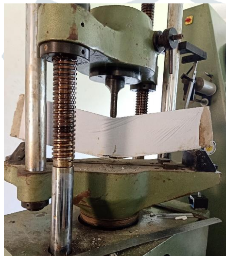
Fig. 3. Flexure test on concrete beam wrapped with waste flex banner
