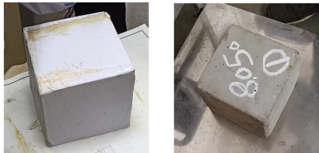
Fig. 2. Wrapped and unwrapped concrete cubes
