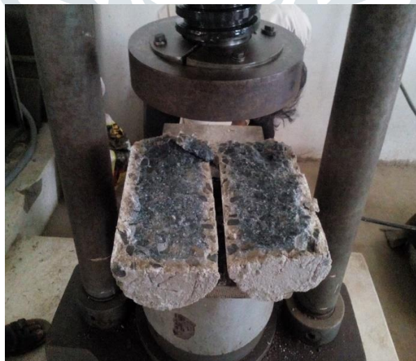
Fig 3: Split Tensile Test specimen after failure.
