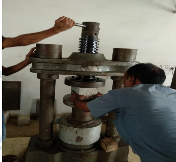
Fig 3.2: Cube testing on compression testing machine
