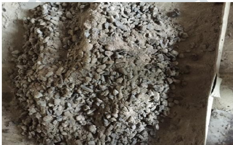
Fig 2: Dry mix of GGBS and aggregates.
