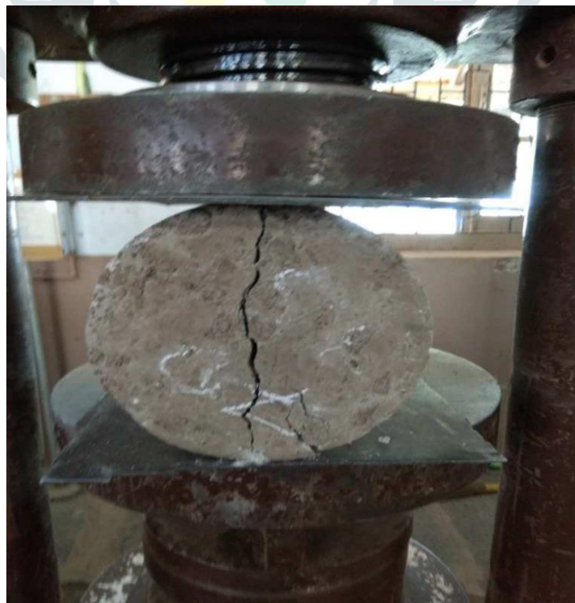
Fig 3.3: Cylinder testing on compression testing machine
