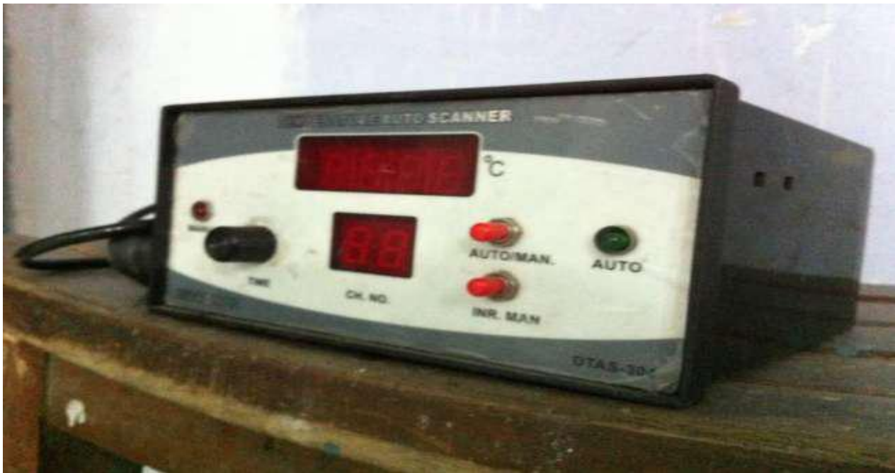
Figure 4.4: Temperature Auto Scanner
