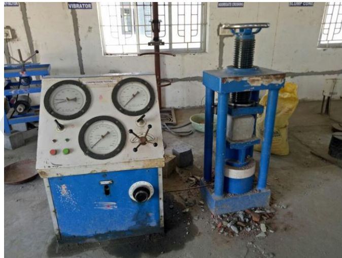
Figure 1 Testing of Concrete Specimens in Compression Testing Machine
