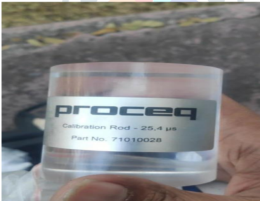
Fig.9- Ultrasonic pulse velocity meter calibration rod
