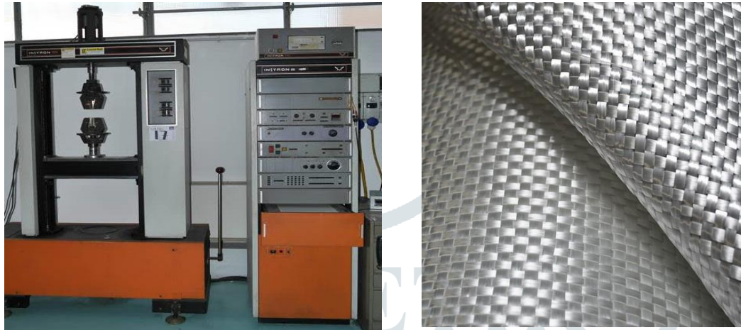
Figure 3 (a): INSTRON 1195 universal testing machine. (b) Glass epoxy woven
