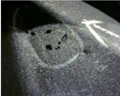
Figure 2.4: Shrinkage and Draw
