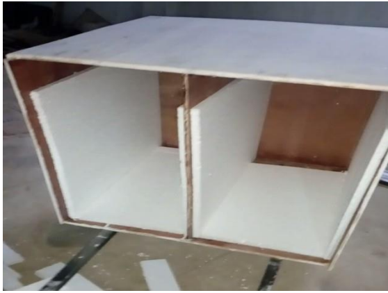
Fig 4 Cooling and heating cabin
