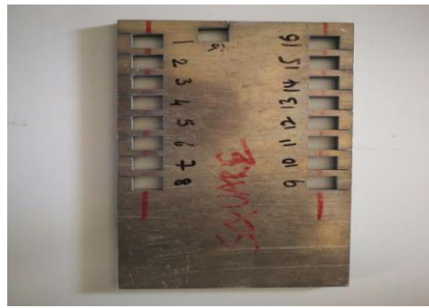
Fig.7: Finally machined square work-pieces for identification of error
