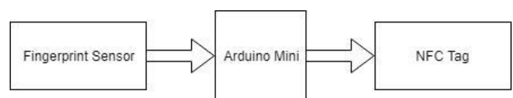
Figure. 2. Block Diagram of NFC Band
