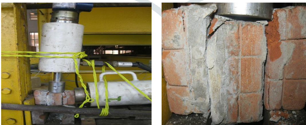
Fig.3: Failure Mechanisms of Masonry Prisms in Shear
