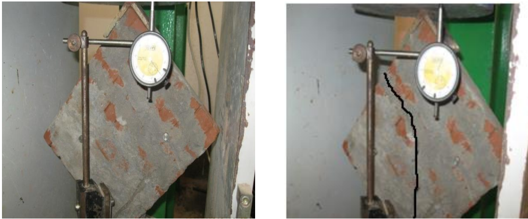
Fig.4: Diagonal Shear Failure Mechanisms of Masonry Prisms
