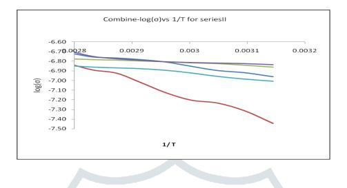
Fig.1- The variation of dc electrical conductivity with temperature (log  $\sigma$ dc Vs 1/T) for all doped polyaniline composite pellet in the temperature range 318 to 358 K.
