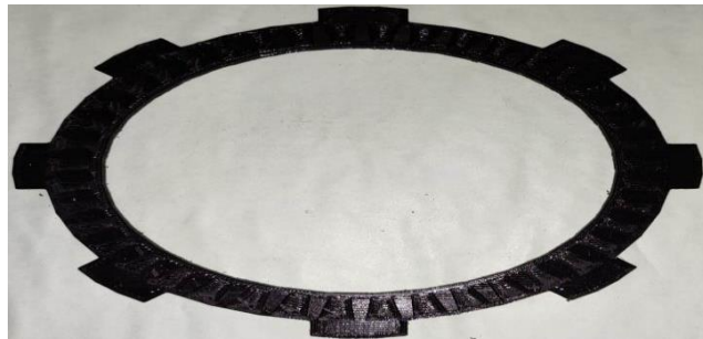
Fig.49. Fusion Deposition Method Taper Profile Plate
