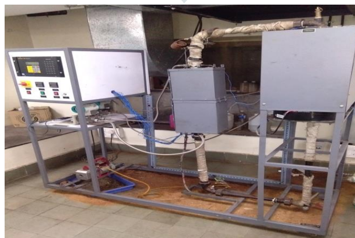
Fig.2 set up of closed loop thermosyphon
