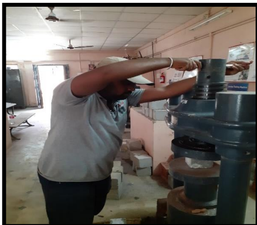
Fig 5.1.1 Compression test of HPC
