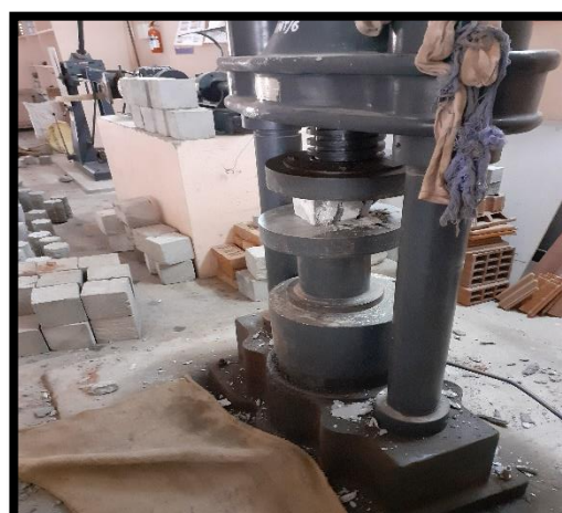
Fig 5.1.2 Compression failure of HPC
