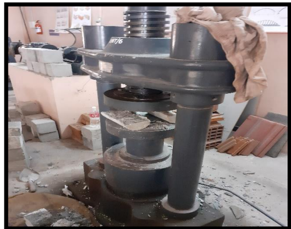
Fig 5.2.2 Split tensile failure of HPC
