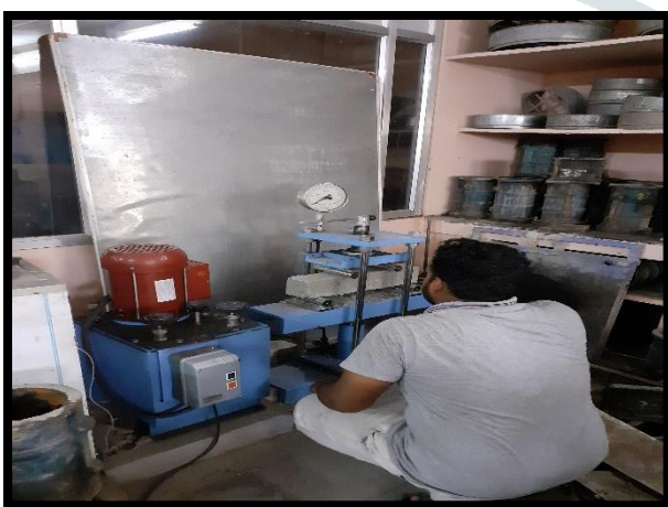
Fig 5.3.1 Flexural strength test of HPC
