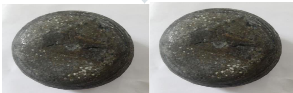
Figure 3.2 Sample of aluminium + Al 2 O 3 7.5 and 10% Alumina in Aluminium
