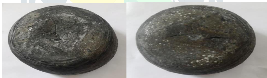
Figure 3.2 Sample of aluminium + Al 2 O 3 7.5 and 10% Alumina in Aluminium
