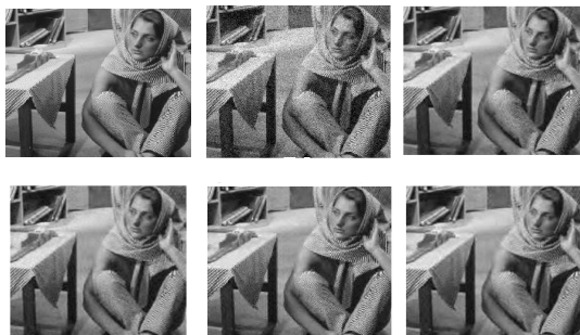
Figure 5.1 (A) Original image, (B) Noisy image (16.11db), (C) Denoise using wavelete (35.27db), (D) Denoise contourlet(SNR=36.03db), (E) In previous method denoise using NSS counterlet transform (SNR=29.83db), (F) in proposed method denoise using NSS counterlet transform(SNR=39.75db)
