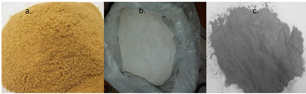
Fig. 1.a.Cork Powder b. Egg shell powder c. Fly ash powder
