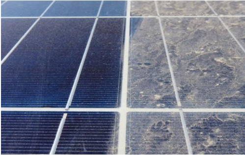
Fig 1. Left - clean panel and right - dusty panel
