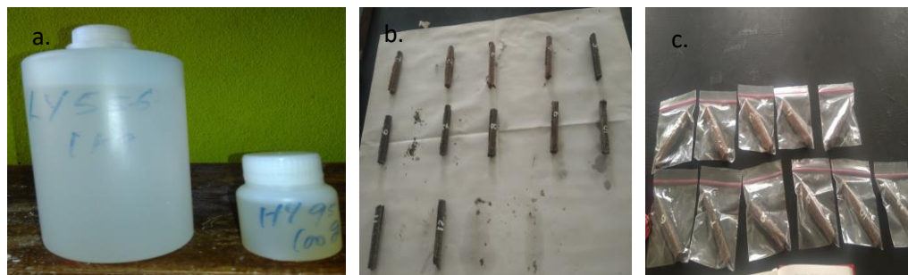
Fig. 2.a.Binder-LY 556, Hardner-HY95 b. Specimens c. Final Specimens after Machining
