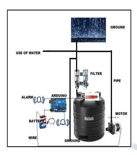
Figure: - INSTALLATION OF SYSTEM
