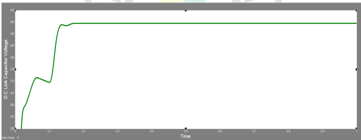
Fig.12- Common D.C Link Capacitor Voltage Waveform
