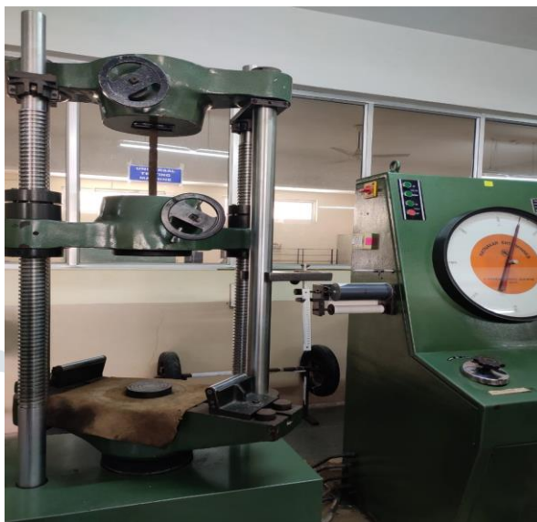
Fig 5.1: Tensile strength test of bamboo
