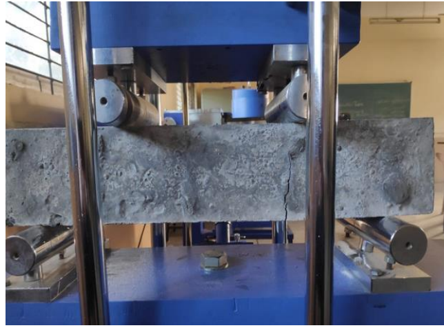
Fig 5.3: Flexural strength of beam
