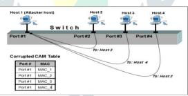
We assume that Host A wants to poison the switch's CAM table, by inserting the invalid entry: MAC address of Host B i.e Switch's Port 0/2 (Fa0/2). This invalid entry will tell the switch that Host B is now located at Port 0/2 (Fa0/2). However, physically, Host B is still located at Port 0/4 (Fa0/4). Hence to perform this attack, Host A should send to any destination host in the LAN network a fake packet (IP or ARP packet) whose Ethernet source MAC address is equal to the MAC address of Host B.
