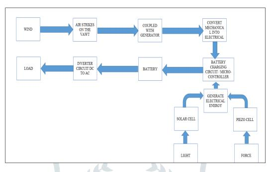
Figure 1.1: Block diagram of the proposed hybrid generation system.
