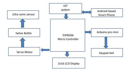
V. FUNCTIONAL DIAGRAM OF HARDWARE ARRANGEMENT OF PROPOSED SYSTEM
