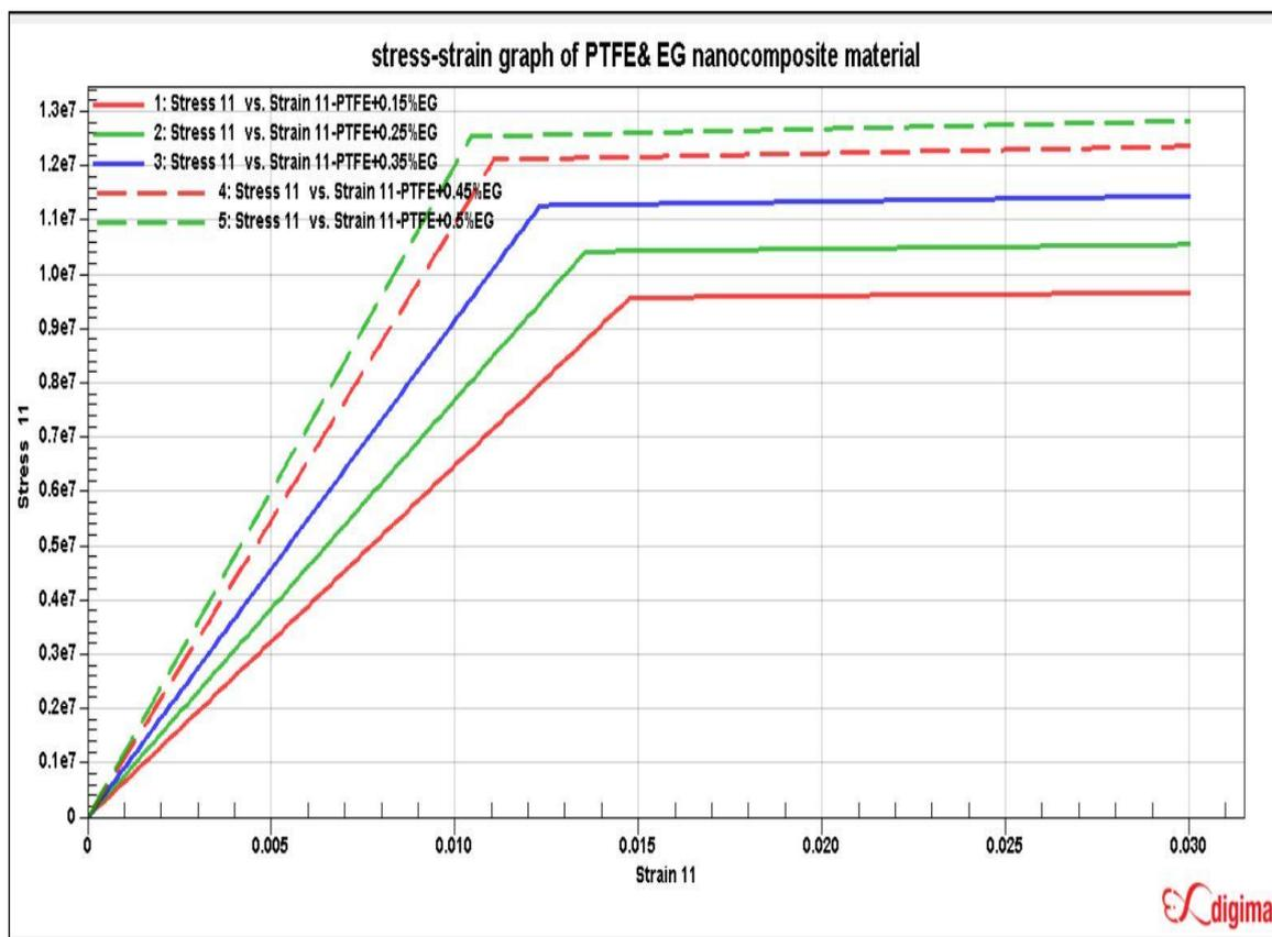
4.2 Stress & strain graph of PTFE & EG nanoparticle in digimat software
