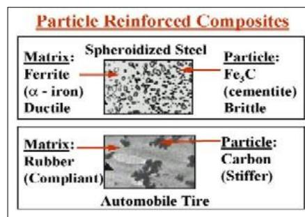
Fig 1.2 Particle reinforced composites
