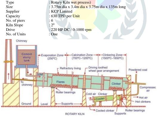
The slurry fed in the Kiln is burnt in to clinker with the heat produced by injecting pulverized fine coal for continuous firing and maintaining temperatures at various zones. The hot clinker coming out from kiln gets cooled, while passing through grate cooler where cold air is passed through cooler grates.
