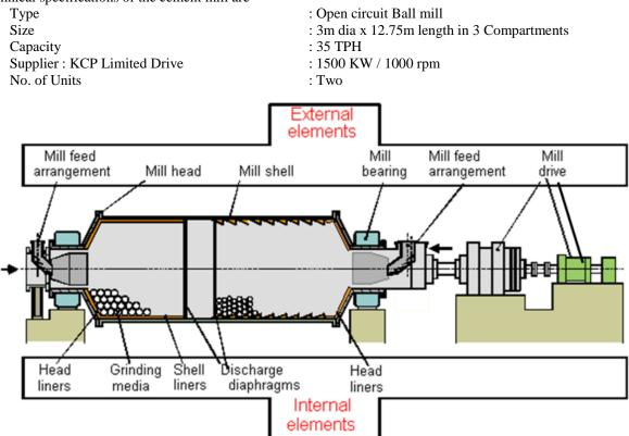
For grinding Ordinary Portland Cement (OPC) a mixture of 95% clinker and 5% Gypsum is fed in to the Mill, whereas for grinding Portland Pozolana Cement (PPC) a mixture of 60% Clinker, 35% Fly ash and 5% Gypsum is fed in to the Mill. The Cement discharged at Cement Mill outlet is conveyed to Cement storage silos with the help of FK Pumps. The venting of Mill is passed through Cyclonic separators and Electro Static Precipitator (ESP) to the stack.
