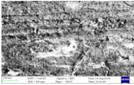
Fig.6 (b) MS sample exposed for 5 h in 1 M HCl
