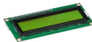
LCD is used to display the data. It acts as an output to microcontroller. It uses ASCII values to display the characters
