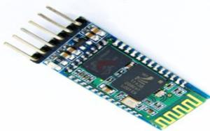
By default the factory setting is SLAVE. The role of this module is to be configured only at commands. SLAVE module cannot initiate a connection to another Bluetooth device but can accept connection.
