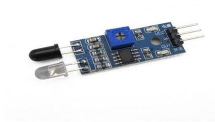
In this project the sensors are placed at some distance from the platform. When the light emitted from the IR LED encounters an object (in this case train) it reflects the light which is picked up by the IR Receiver. The desired operation is performed when the light reflects from the object (in this case opening/closing the mobile platform)
