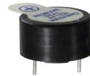
A piezoelectric diaphragm consists of a piezoelectric ceramic plate which has electrodes on both sides and a metal plate (brass or stainless steel, etc.). A piezoelectric ceramic plate is attached to a metal plate with adhesives. Applying D.C. voltage between electrodes of a piezoelectric diaphragm causes mechanical distortion due to the piezoelectric effect
