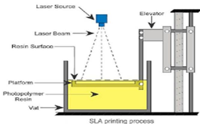
Stereolithographic 3D Printing Fig.2
