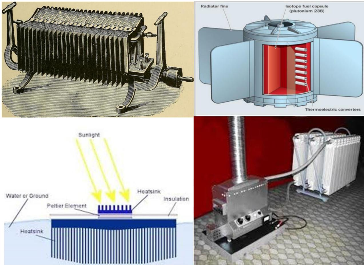
**Fig 6. : Thermoelectric generator**
