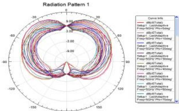
Figure 2: Radiation Pattern of H-shaped
