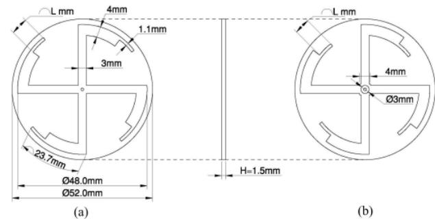
Figure 1. Geometrical structure presentation of the proposed antenna (a) top view (b) bottom view
