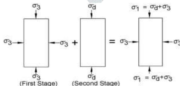
Fig. 4. Cylindrical specimen subjected to stresses in CU test
