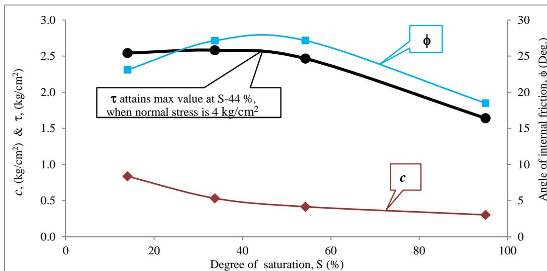
Fig. 9. Variation of shear strength parameters with degree of saturation
