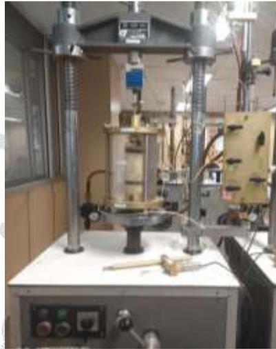
Fig. 3. Semi-automatic triaxial machine
