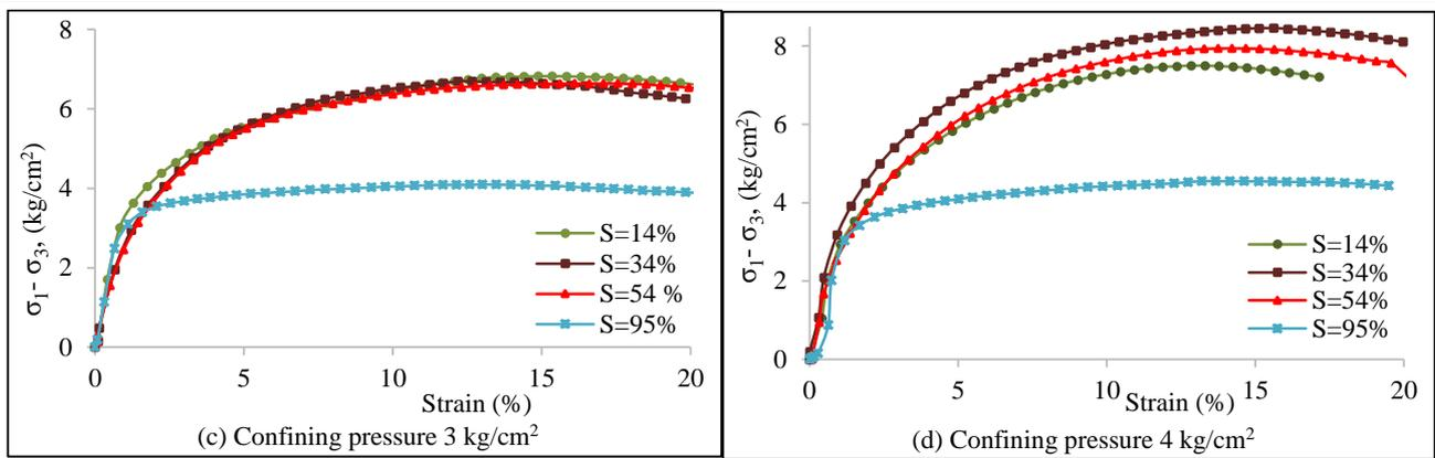
**Fig. 7.** Deviator stress-strain graph for different samples at confining pressures of (a) 1 kg/cm<sup>2</sup> (b) 2 kg/cm<sup>2</sup> (c) 3 kg/cm<sup>2</sup> and (d) 4 kg/cm<sup>2</sup>.
