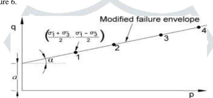
Fig. 6. Modified failure envelope, (p-q plot)
