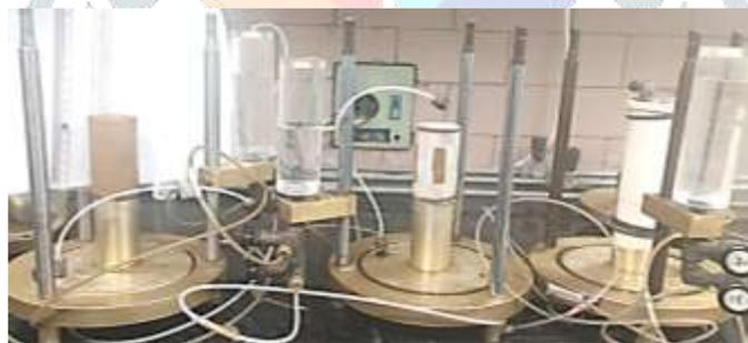
**Fig. 2.** Preparation of specimen in triaxial cell apparatus
