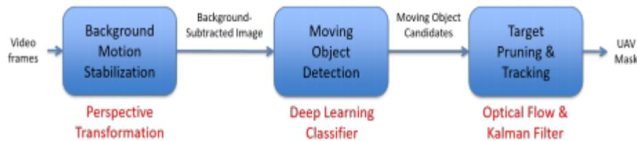
Fig 1. Moving Object Detection and Tracking process.
