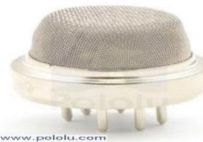
This semiconductor MQ02 sensor detects the presence of combustible CO<sub>2</sub> along with smoke at concentrations. These are easy to install and are used in both residential as well as commercial sectors. If any CO<sub>2</sub> is detected by the sensor then it is going to alert the micro controller.
