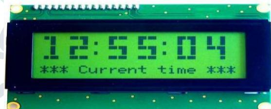
One of the most common devices attached to a micro controller is an 16x2 LCD display. This means 16 characters per line by 2 lines and 20 characters per line by 2 lines, respectively. The project status will display on LCD.
